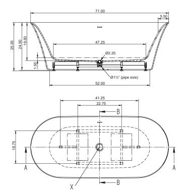
Product measure tolerances  $\pm \frac{1}{2}$ ". Frame location tolerance according to X  $\pm 1$ "
