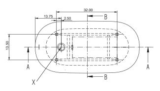
Product measure tolerances  $\pm \frac{1}{2}$ ". Frame location tolerance according to X  $\pm 1$ "
