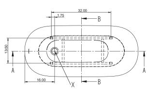
Product measure tolerances  $\pm \frac{1}{2}$ ". Frame location tolerance according to X  $\pm 1$ "
