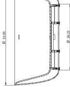
Product measure tolerances  $\pm 1\!/\!2$  ". Frame location tolerance according to X  $\pm 1$  "
