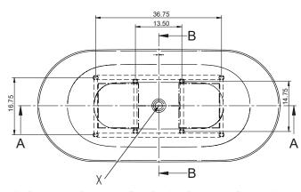
Product measure tolerances  $\pm \frac{1}{2}$ ". Frame location tolerance according to X  $\pm 1$ "
